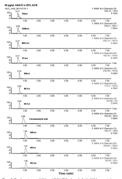
Figure 2. The chromatogram of HAAs on HILIC UPLC column (individual HAA concentration was 50 pg/ $\mu$ L, injection 30  $\mu$ L).
