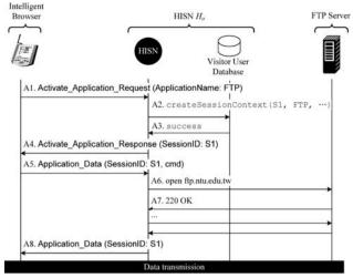
Fig. 8 The message flow for the application activation procedure
