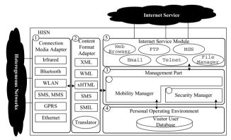
Fig. 3 The software architecture of an HISN
