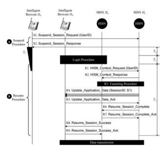
Fig. 9 The message flow for the suspend and resume procedures
