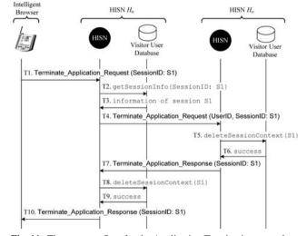
Fig. 11 The message flow for the Application Termination procedure
