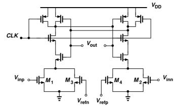
respectively. Assume  $V_{in}$  has common-mode voltage at  $V_{cm}$  and  $V_{rcm}$  and  $M_1-M_4$  are in linear region when CLK is low. Identify the characteristics of the comparator and determine if we need to have the same  $V_{cm}$  and  $V_{rcm}$  to allow the circuit work properly.
