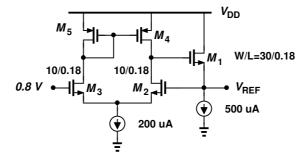
(Hint:  $M_4$  has to be in saturation region) by simulation. What is the small-signal output impedance of the circuit? What would this suggest about the worst-case settling time of the above DAC if it uses this reference?
