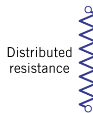
(a) Resistance distributed between two terminals
