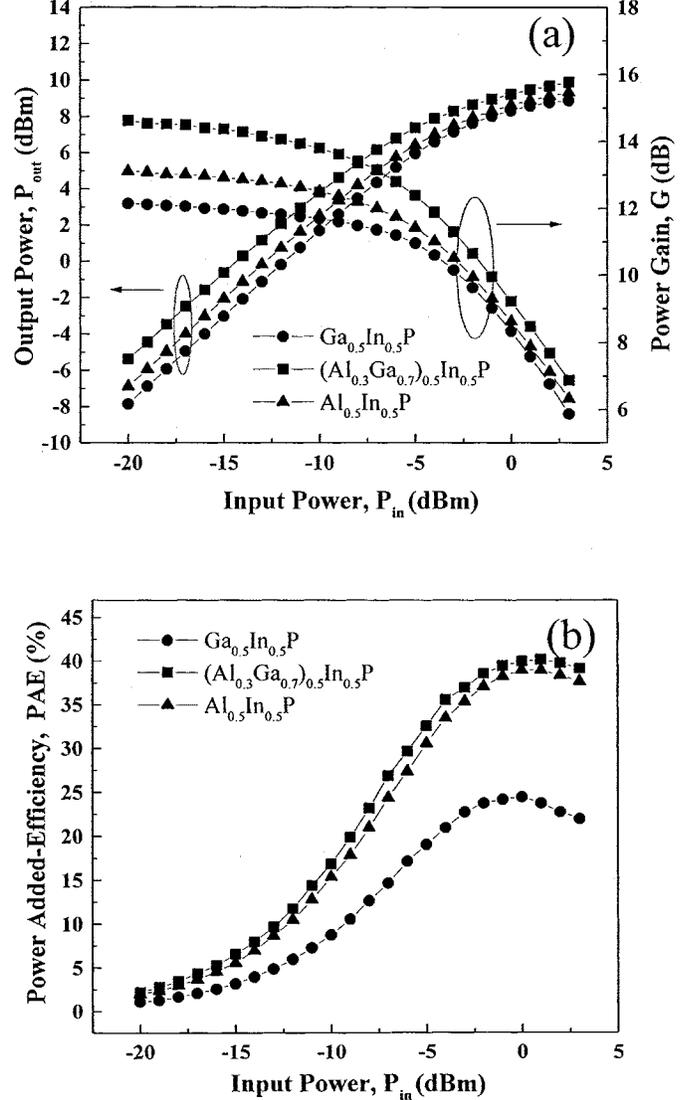
Fig. 6. Power performance of  $(\text{Al}_x\text{Ga}_{1-x})_{0.5}\text{In}_{0.5}\text{P}/\text{In}_{0.15}\text{Ga}_{0.85}\text{As}$  DCFETs with a gate length of  $1.0 \mu\text{m}$  at  $1.9 \text{ GHz}$  ( $V_{\text{DS}} = 3.0 \text{ V}$ ): (a) output power and power gain versus input power and (b) power added efficiency (PAE) versus input power.
