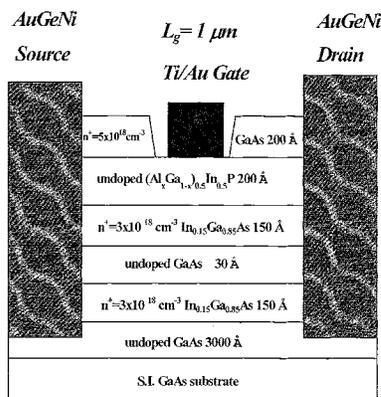
Fig. 1. Device cross section of  $(\text{Al}_x\text{Ga}_{1-x})_{0.5}\text{In}_{0.5}\text{P}/\text{In}_{0.15}\text{Ga}_{0.85}\text{As}$  ( $x = 0, 0.3, 1.0$ ) DCFETs.
