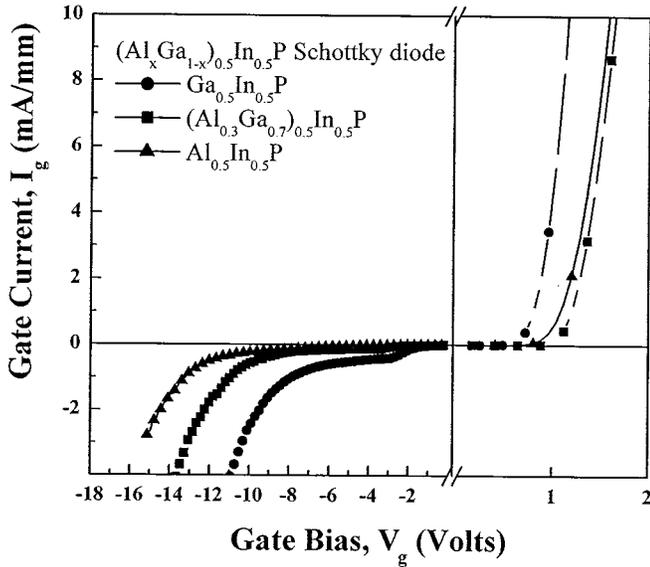
Fig. 3. Schottky diode  $I$ - $V$  characteristics for different  $x$  values of  $(\text{Al}_x\text{Ga}_{1-x})_{0.5}\text{In}_{0.5}\text{P}$  compounds.
