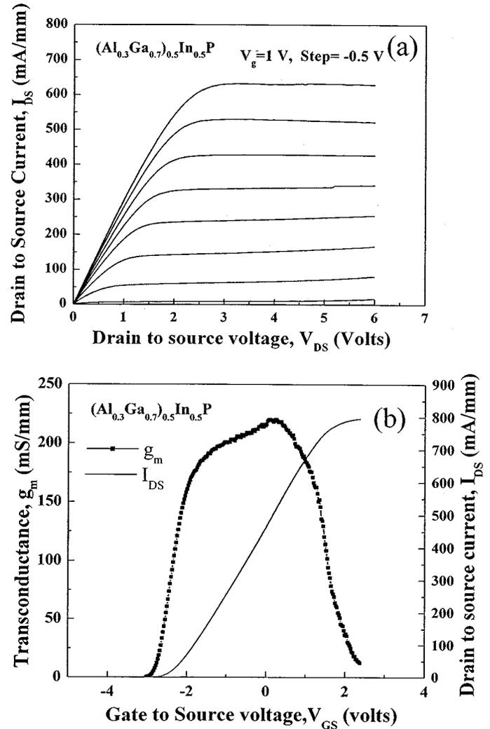
Fig. 4. DC  $I$ - $V$  characteristics of  $(\text{Al}_{0.3}\text{Ga}_{0.7})_{0.5}\text{In}_{0.5}\text{P}/\text{In}_{0.15}\text{Ga}_{0.85}\text{As}$  DCFETs with a gate-length of  $1.0 \mu\text{m}$ : (a)  $I_{\text{DS}}-V_{\text{DS}}$  curves, and (b)  $g_m-I_{\text{DS}}-V_{\text{GS}}$  transfer curves.
