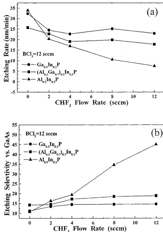
Fig. 2. (a) RIE etching rates and (b) selectivities versus GaAs of various  $(\text{Al}_x\text{Ga}_{1-x})_{0.5}\text{In}_{0.5}\text{P}$  quaternary compounds versus  $\text{CHF}_3$  flow rates at a  $\text{BCl}_3$  flow rate of 12 sccm.
