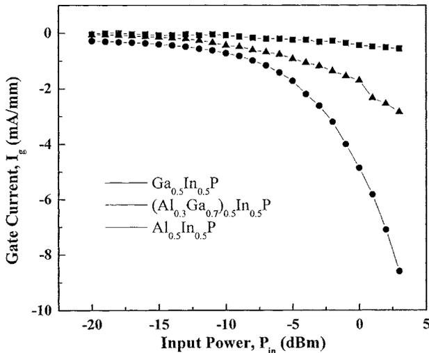
Fig. 7. Gate leakage current versus input power of  $(\text{Al}_x\text{Ga}_{1-x})_{0.5}\text{In}_{0.5}\text{P}/\text{In}_{0.15}\text{Ga}_{0.85}\text{As}$  ( $x = 0, 0.3, 1.0$ ) DCFETs for  $1.0 \mu\text{m} \times 50 \mu\text{m}$  devices.
