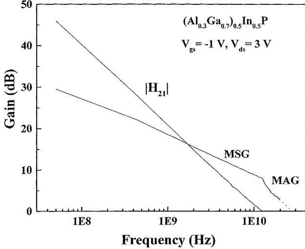
Fig. 5. Microwave characteristics of  $(\text{Al}_{0.3}\text{Ga}_{0.7})_{0.5}\text{In}_{0.5}\text{P}/\text{In}_{0.15}\text{Ga}_{0.85}\text{As}$  DCFETs with a gate length of  $1.0 \mu\text{m}$  and a width of  $50 \mu\text{m}$ .
