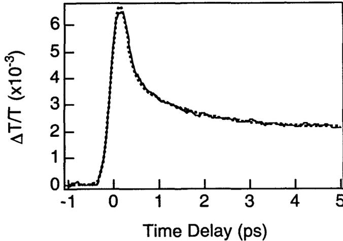
Figure 2. Measured transient absorption saturation at a wavelength of 370 nm. The dotted line is a convolution fit.
