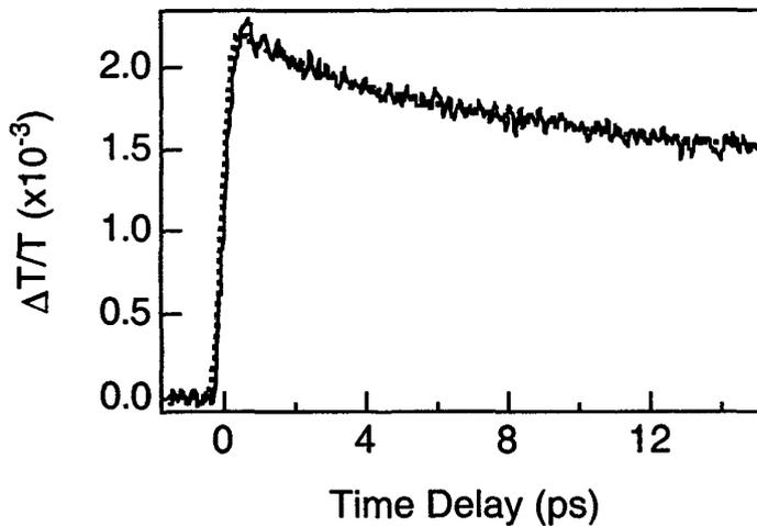
Figure 3. Measured transient absorption saturation at a wavelength of 374 nm. The dotted line is a convolution fit.
