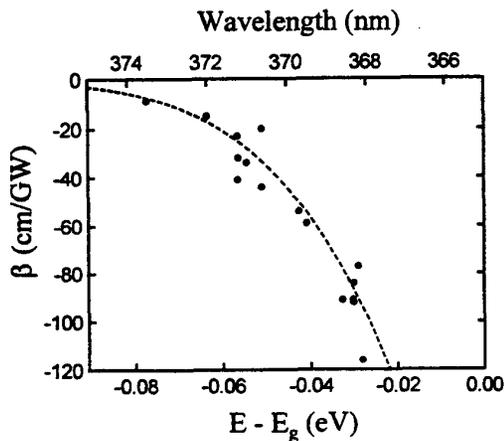
Figure 1. Measured absorption saturation versus wavelength using open aperture Z-scan techniques. The dotted line is a fit.
