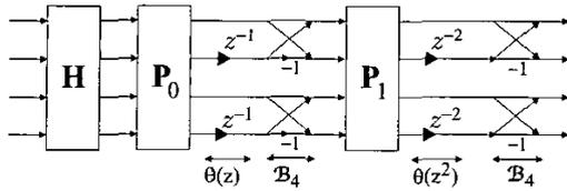
Figure 1: A  $4 \times 4$  lapped Hadamard matrix  $E_2(z)$  constructed by the butterfly method.
