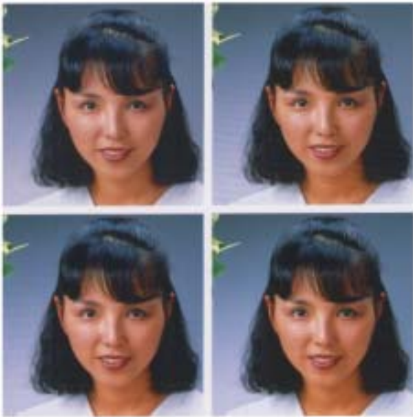
Figure 11. 4 halftone images with 100, 133, 175, 150 LPIs starting from the left-upper corner in the clockwise direction scanned at 100 dpi.
