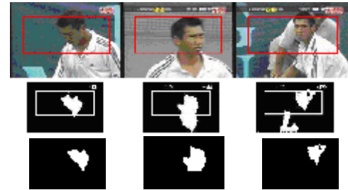
Fig.7 Illustration of face detection: first row: close-up scene; second row: depicts the skin color distribution; third row: depicts the region considered as face region.
