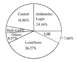
Figure 13. The pie chart of Compress's execution cycle time.
