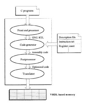
Figure 6. The prototype of compiler in FACE.
