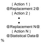
The macro expression defines the functions that will be expanded in other entries, thus shrinking the redundancy. The replacement option is used to satisfy the design goal as accurately as possible and triggered by tuning box's rule engine to make a suitable decision. Actions are the output object code for this rule. If one of the replacement rules is selected, the corresponding action will be output. The statistical data is for partitioning hardware and software.
