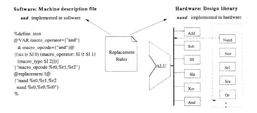
Figure 12. The replacement between hardware/software for logical operators, and, nand.
