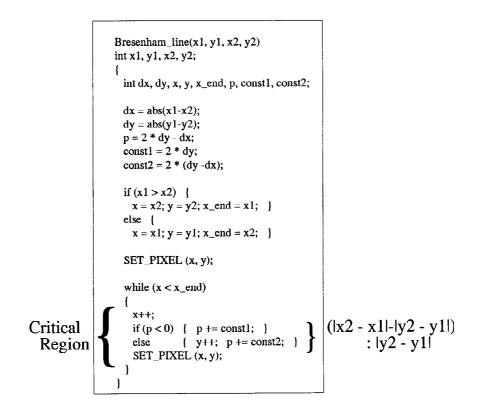
Figure 14. Bresenham's line-drawing algorithm in C.
