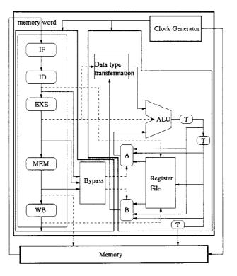
Figure 11. The block diagram for the modified DLX.
