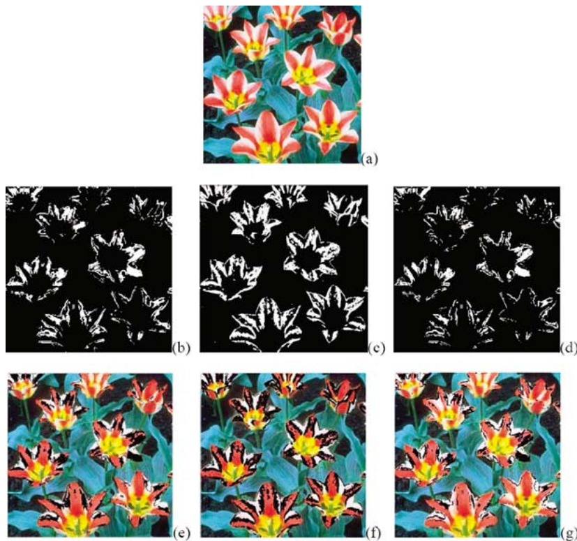
Fig. 15. Color-sensitive edge detection between two selected colors for a natural image. The selected two red and white colors are (237, 157 157) and (255, 255, 255). (a) Natural image. (b) Horizontal and vertical edges detected by RBs. (c) Horizontal and vertical edges detected by conventional quaternions in [10]. (d) Diagonal edges detected by RBs. (e) Combination of the natural image and the negative of (b). (f) Combination of the natural image and the negative of (c). (g) Combination of the natural image and the negative of (d). (Black pixels shown in (e)–(g) have been identified as either horizontal-vertical or diagonal, red-white or white-red, or edge pixels.)
