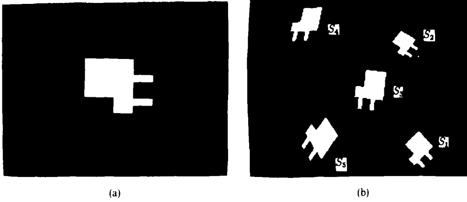
Fig. 10. (a) Monocular tracking test: R_{ref} : placed at (0, 0, 1) , orientation at (0, 0, -1) . (b) Different R_{obs} .
