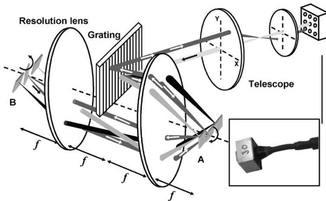
Fig. 9. Schematic setup of the  $1 \times N^2$  WSS with a monolithic 2-D collimator array. The telescope is used to expand the beam size.
