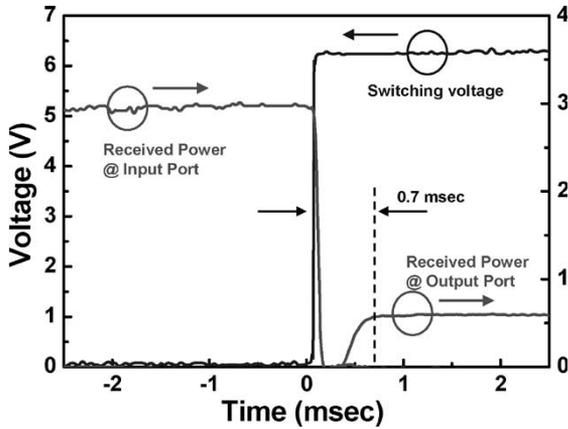
Fig. 11. Measured switching time of the wavelength-selective  $1 \times N^2$  switch.
