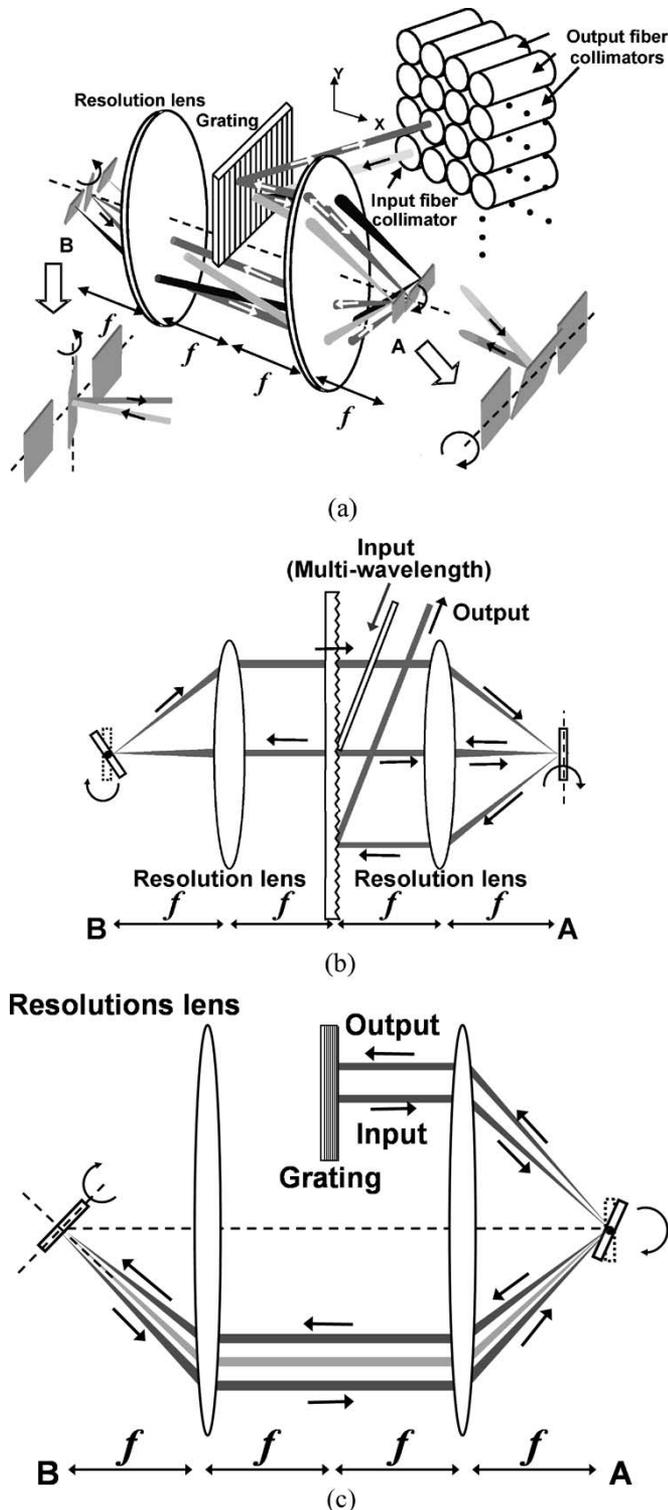
Fig. 3. (a) Schematic setup of the  $1 \times N^2$  WSS. The two orthogonally scanning micromirror arrays enable the fibers to be arranged in two dimensions, which increases the output port from  $N$  to  $N^2$ . (b) Top view of the  $1 \times N^2$  WSS. (c) Side view of the  $1 \times N^2$  WSS.
