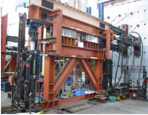
Figure 1. Test setup of the friction coefficient test
