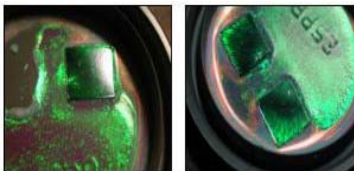
Fig. 6 Three-dimensional PBG crystals prepared from 260 nm silica spheres.
