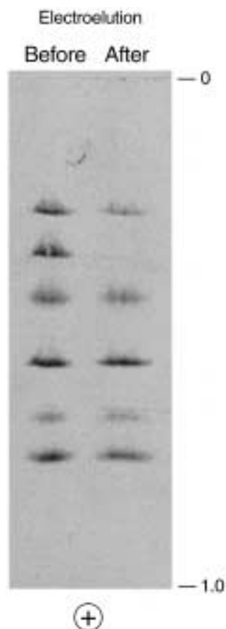
Figure 2. PhastSystem SDS-PAGE electropherogram of the mixture of six standard proteins before and after electroelution of the BSA band. PhastSystem 8–25%T pore gradient gel, operative pH 8.06, ionic strength 0.042, 15°C.
