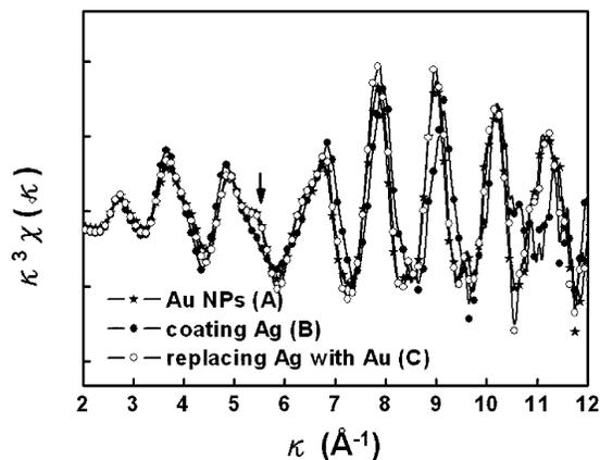
**Figure 2.** Au  $L_3$  edge EXAFS oscillations for Au nanoparticles (a), Au colloids whose surfaces were coated with shells of pure silver (b), and  $\text{Au}_{\text{core}}\text{Ag}_{\text{shell}}$  nanoparticles in which Ag was replaced with  $\text{HAuCl}_4$  (0.4 mL) solution (c). The arrow indicates oscillation caused by the presence of Ag.
