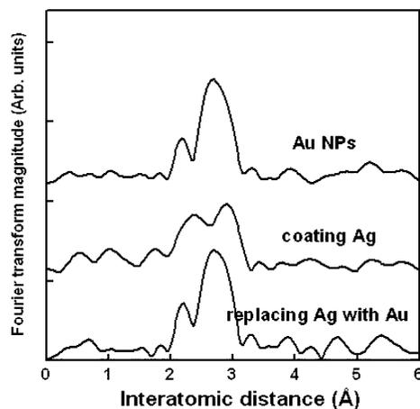
**Figure 3.** EXAFS analysis of Au nanoparticles, Au colloids whose surfaces have been coated with shells of pure silver, and  $\text{Au}_{\text{core}}\text{Ag}_{\text{shell}}$  nanoparticles in which Ag was replaced with  $\text{HAuCl}_4$  (0.4 mL) solution. Fourier transforms of Au  $L_3$  edge  $k^3\chi(k)$  EXAFS spectrum of product in each reaction step.
