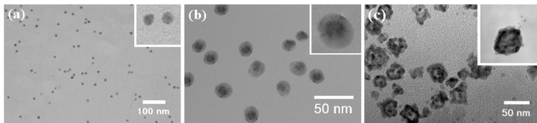
**Figure 1.** (a) TEM image of Au nanoparticles. (b) TEM image of Au colloids whose surfaces have been coated with shells of pure silver. (c) TEM image of nanorattles that had been prepared by adding  $\text{HAuCl}_4$  solution to the colloids from part b.
