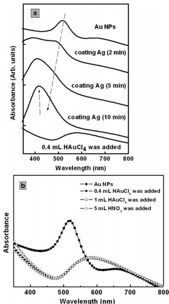
**Figure 5.** (a) Extinction spectra obtained by adding  $\text{AgNO}_3$  solution to the Au nanoparticles in various stages; 0.4 mL of  $\text{HAuCl}_4$  solution was added to Au NPs coated with Ag shell. Time evolves from 0 to 10 min. (b) UV-vis extinction spectra of as-prepared nanorattles after  $\text{HAuCl}_4$  and  $\text{HNO}_3$  solutions were added.
