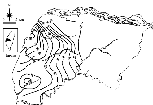
Fig. 3. The contour of cumulative land subsidence from 1985 to 1994 (units in cm, adapted from Du et al., 1996).
