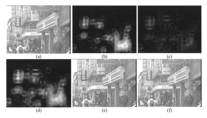
Fig. 2. An example of the road-sign detection process. (a) Original input image. (b) Color feature map of input image. (c) Shape feature map of the input image. (d) Integration map of color and shape features. (e) Result after the integration step. (f) Result after the verification step.
