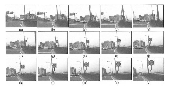
Fig. 10. Experimental results with video sequence  $S_1$ . The first 15 frames of this sequence are shown in (a) to (o). The size of each image is  $320 \times 240$  pixels and the time between two successive images is 0.2 s.
