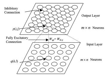
Fig. 3. Sketch of the neural network for color (or shape) feature detection, where (i, j) is the position of neuron p on the output layer, (k, l) is the position of neuron q on the input layer, and  $w_{kl,ij}$  is the weight between neurons q and p.
