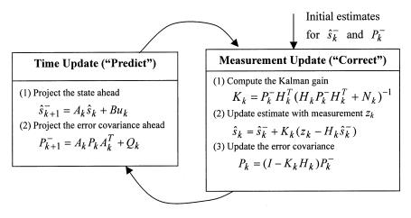
Fig. 8. Operation of the Kalman filter [16].
