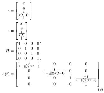
where f is the focal length of the camera, v is the vehicle velocity,  $R_r$  is the radius of the road sign, and  $\Delta t$  is the time interval for updating.
