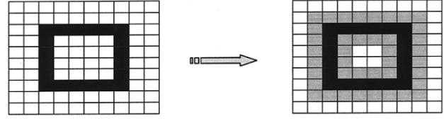
Fig. 2. Watermark processed with 3 \times 3 morphological dilation.
