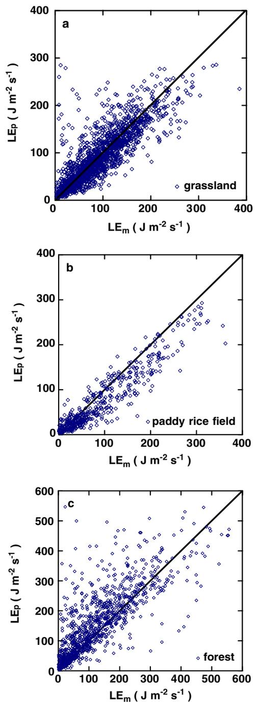
**Fig. 12** Comparisons of eddy-covariance measured ( $LE_m$ ) and flux-variance predicted ( $LE_p$ ) water vapor fluxes for **a** grassland, **b** rice paddy field, and **c** forest with  $LE_p$  estimated by Eq. (10) with measured sensible heat flux. The 1:1 line is also shown
