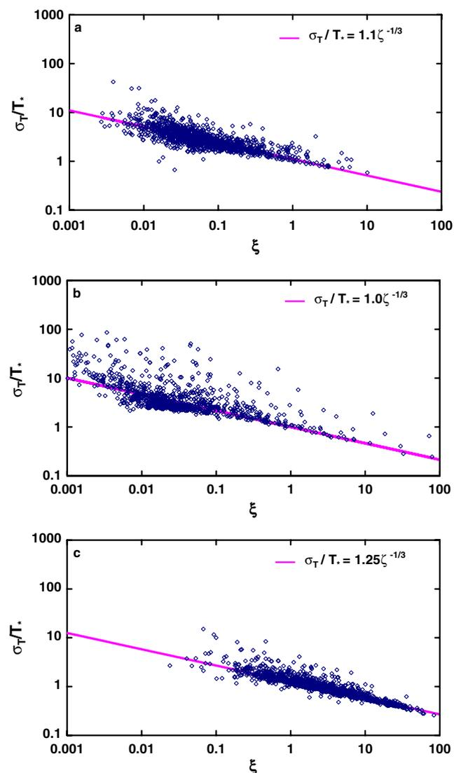
**Fig. 7** Normalized standard deviation of temperature ( $\sigma_T/T_*$ ) as a function of stability parameter ( $\xi$ ) for **a** grassland, **b** rice paddy field, and **c** forest
