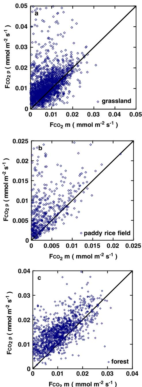
**Fig. 13** Comparisons of eddy-covariance measured ( $F_{CO_2m}$ ) and flux-variance predicted ( $F_{CO_2p}$ )  $CO_2$  fluxes for **a** grassland, **b** rice paddy field, and **c** forest. The 1:1 line is also shown
