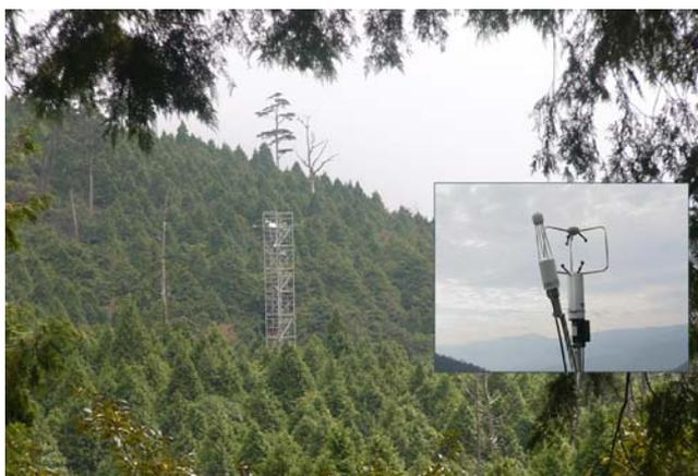
**Fig. 3** Experimental set-up for the forest Site
