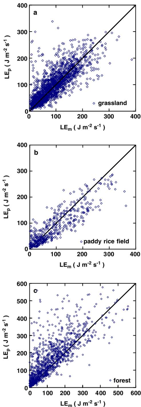
**Fig. 11** Comparisons of eddy-covariance measured ( $LE_m$ ) and flux-variance predicted ( $LE_p$ ) water vapor fluxes for **a** grassland, **b** rice paddy field, and **c** forest. The 1:1 line is also shown
