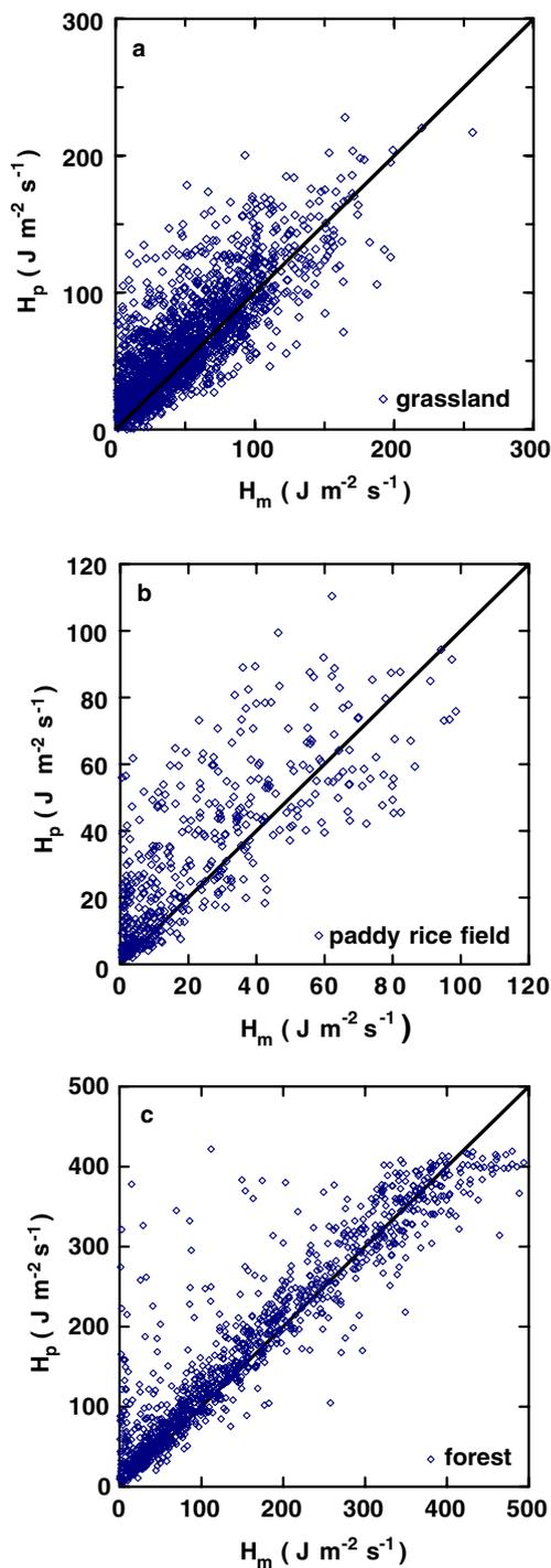
**Fig. 10** Comparisons of eddy-covariance measured ( $H_m$ ) and flux-variance predicted ( $H_p$ ) sensible heat fluxes for **a** grassland, **b** rice paddy field, and **c** forest. The 1:1 line is also shown
