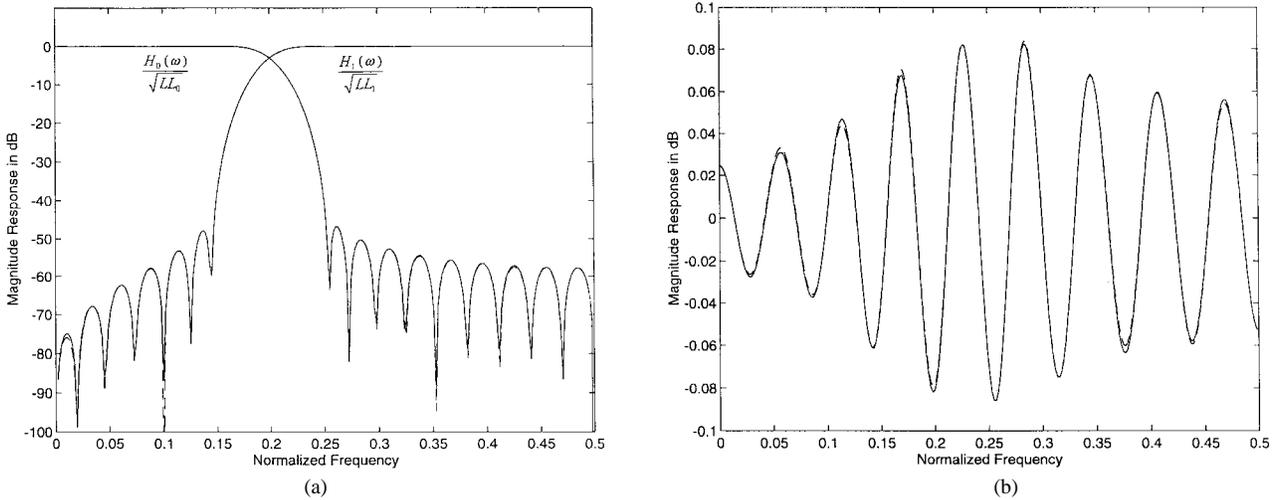
Fig. 4. Magnitude responses for Example 1. (a)  $H_0(\omega)/\sqrt{LL_0}$  and  $H_1(\omega)/\sqrt{LL_1}$ . (b)  $T(\omega)$ .
