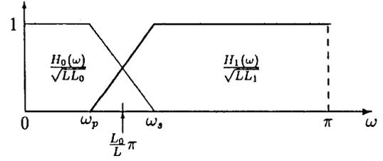
Fig. 2. Desired magnitude specifications for the analysis filters.
