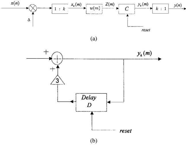
Fig. 3. Proposed new filter structure. (b) Function block C.
