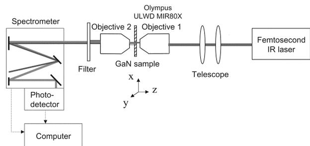
FIG. 3 Experimental layout for the scanning second- and third-harmonic generation (SHG/THG) microscopy of GaN. IR = infrared.
