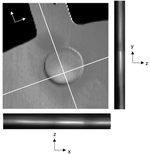
FIG. 10 x-z, y-z, and their corresponding x-y scanned second-harmonic generation images of the bulk GaN sample. The white lines on top of the x-y image indicate the positions of the z-directional scans.
