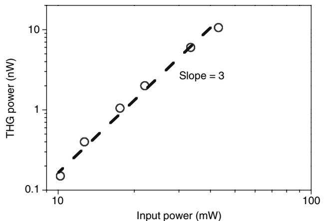
FIG. 7 Average third-harmonic generation (THG) power versus average input infrared power in a 2.5  $\mu\text{m}$  thick GaN sample. The experiment was performed with an 80 $\times$  objective. The open circles are experimental data and the dashed line is a guided line with a slope of 3.
