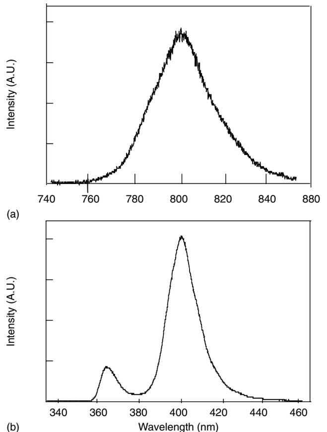
FIG. 12 (a) Fundamental infrared spectrum of the Ti:sapphire centered at 800 nm and (b) the excited nonlinear spectrum after the InGaN multiple quantum well sample. The symmetric spectrum centered at 400 nm is the generated second-harmonic generation. The luminescence peak centered at 365 nm corresponds to the three photon-induced bandedge photoluminescence from the GaN substrate. A.U. = arbitrary unit.
