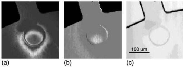
FIG. 8 (a) Scanning third-harmonic generation image, (b) scanning second-harmonic generation image, and (c) their corresponding transmission image of a GaN Hall-measurement sample. The transmission image was taken with the fundamental infrared beam.
