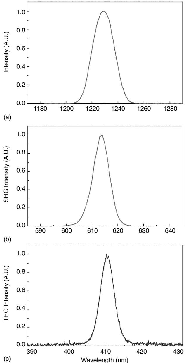
FIG. 4 Spectra for (a) infrared (IR) laser beam, (b) second-harmonic generation (SHG), and (c) third-harmonic generation (THG) signals from a 2.5  $\mu\text{m}$ -thick bulk GaN. The IR laser output from a femtosecond Cr:forsterite laser was centered at 1230 nm, while the SHG and THG spectra are centered at 615 nm and 410 nm respectively. A.U. = arbitrary unit.
