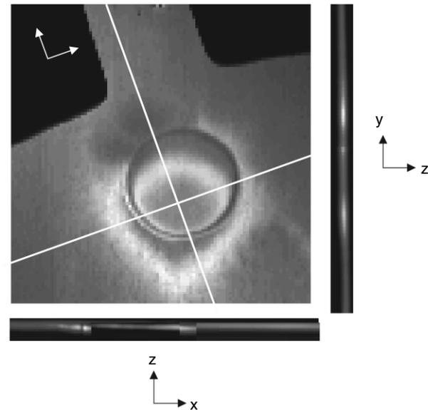
FIG. 11 x-z, y-z, and their corresponding x-y scanned third-harmonic generation images of the bulk GaN sample. The white lines on top of the x-y image indicate the positions of the z-directional scans.
