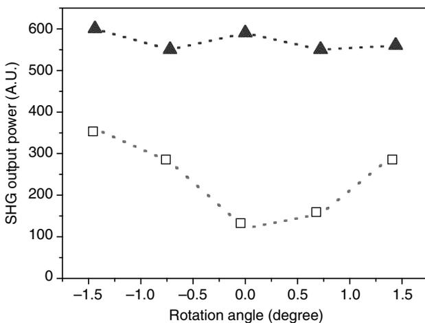
FIG. 5 Angle-dependent second-harmonic generation (SHG) powers on the bulk GaN sample with an 80 $\times$  and a 50 $\times$  objective.
