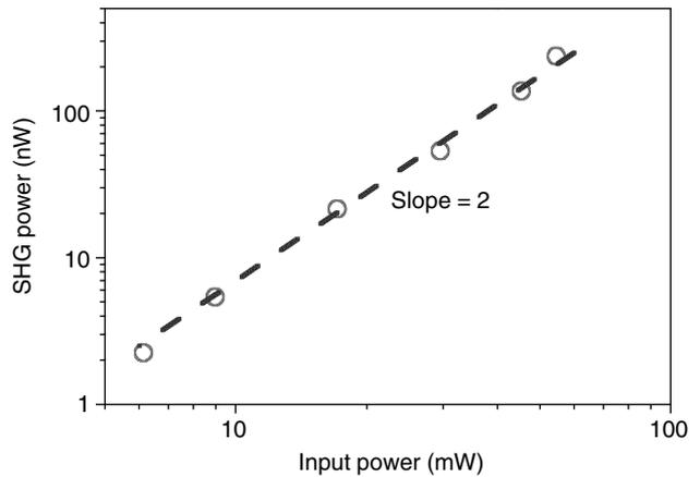
FIG. 6 Average second-harmonic generation (SHG) power versus average input infrared power in a 2.5  $\mu\text{m}$  thick GaN sample. The experiment was performed with an 80 $\times$  objective. The open circles are experimental data and the dashed line is a guided line with a slope of 2.
