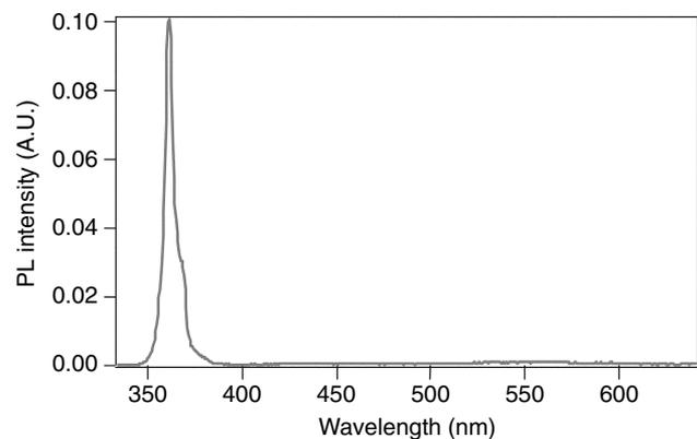
FIG. 1 Photoluminescence (PL) spectrum of a bulk GaN sample excited by a continuous-wave (CW) HeCd laser. Luminescence peak at 365 nm (3.39 eV) corresponds to bandedge emission. Below the bandgap luminescence, a weak bandtail luminescence between 365 and 390 nm and a weak yellow luminescence centered at 550 nm can be observed. A.U. = arbitrary unit.
