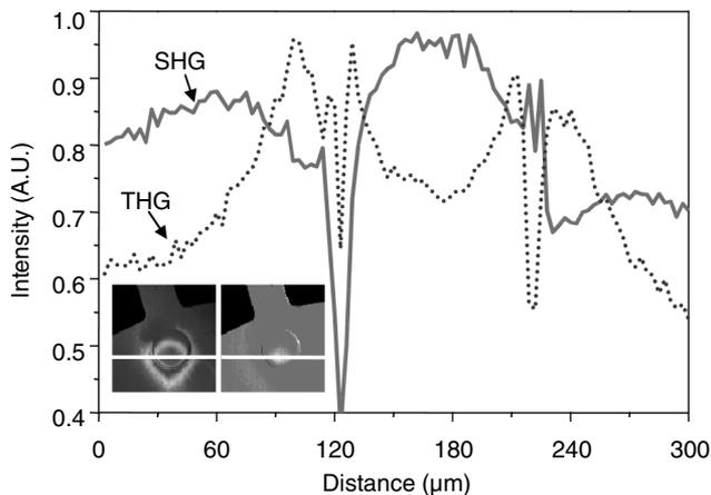
FIG. 9 Linescan of the second-harmonic generation intensity and its corresponding third-harmonic generation intensity across the oval defect in a GaN sample. The position of the performed linescan is shown in the inset. A.U. = arbitrary unit.
