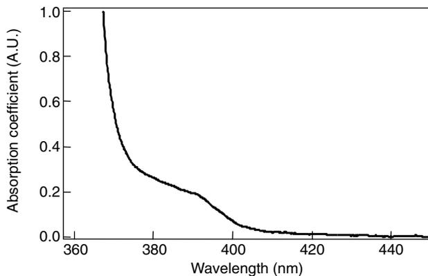
FIG. 2 Absorption spectrum of an InGaN multiple quantum well (MQW) sample with 1.2 nm wellwidth. The rise of the absorption of approximately 395 nm (3.14 eV) corresponds to the MQW bandgap transition energy. The sharp rise of the absorption at 365 nm is due to the absorption in the GaN substrate underneath. A.U. = arbitrary unit.
