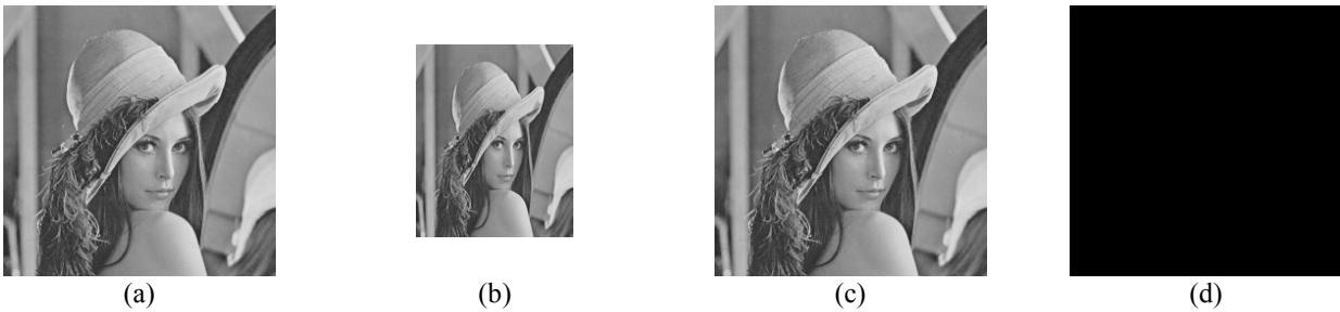
Fig.4 (a) Original input image. (b) Down sampled image in the upper channel. (c) Perfectly reconstructed output image. (d) Reconstruction error.
