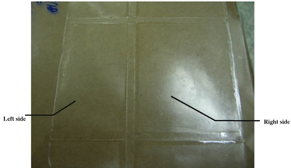
Fig. 5. A PET substrate with stamped polymeric microlens array.
