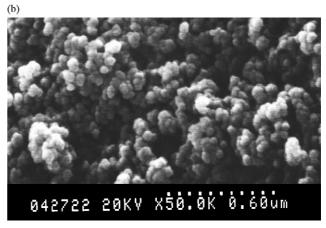
Fig. 3. Scanning electron micrographs of (a)  $TiO_2$  and (b) Ag/TiO<sub>2</sub> (50,000×).
