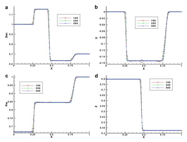
Fig. 2. Test of the grid convergence of gas-kinetic QBGK scheme (NS2): (a) number density; (b) mean velocity; (c) pressure; (d) fugacity.
