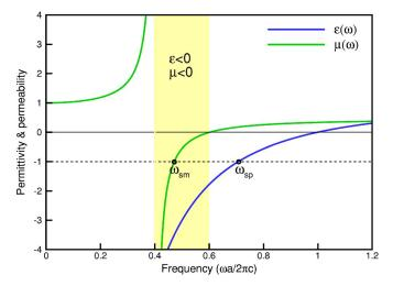
FIG. 1. (Color online) The effective  $\varepsilon$  and  $\mu$  of the negative index material for  $\omega_p a/2\pi c = 1.0$ ,  $\omega_0 a/2\pi c = 0.4$ , and F = 0.56. The yellow region corresponds to the frequency range where the medium has both negative  $\varepsilon$  and  $\mu$ . The black circles denote the locations of  $\omega_{\rm sp}$  and  $\omega_{\rm sm}$  for  $\varepsilon_d = 1$  and  $\mu_d = 1$ .
