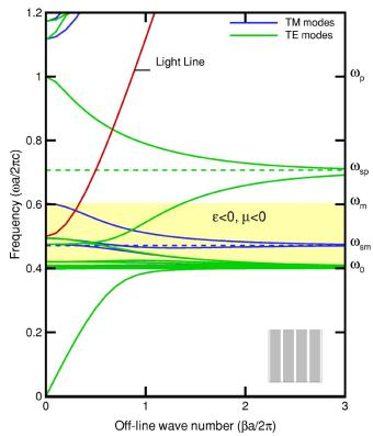
FIG. 3. (Color online) The dispersion relations at  $ka/2\pi=0.5$  for a one-dimensional layered structure of negative index material of thickness t/a=0.8 where  $\omega_p a/2\pi c=1.0$ ,  $\omega_0 a/2\pi c=0.4$ , and F=0.56.
