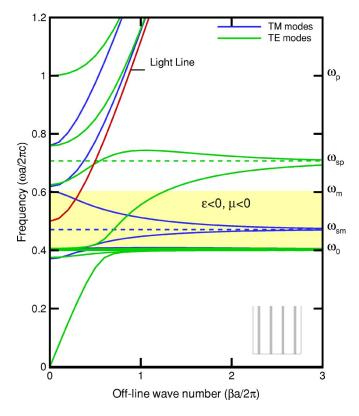
FIG. 2. (Color online) The dispersion relations at  $ka/2\pi=0.5$  for a one-dimensional layered structure of negative index material of thickness t/a=0.2 where  $\omega_p a/2\pi c=1.0$ ,  $\omega_0 a/2\pi c=0.4$ , and F=0.56.
