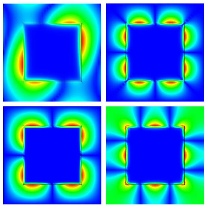
FIG. 14. (Color online) Four typical AS modes in magnitude for TE polarization with frequencies near  $\omega_0$  at the point  $\Gamma$  for a square array of square cylinders of negative index material of half-width w/a=0.3 where  $\omega_p a/2\pi c=1.0$ ,  $\omega_0 a/2\pi c=0.4$ , and F=0.56.
