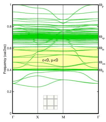
FIG. 10. (Color online) The TE band structures for a square array of grid cylinders of negative index material with the thickness ratio t/a=0.1, where  $\omega_p a/2\pi c=1.0$ ,  $\omega_0 a/2\pi c=0.4$ , and F=0.56.
