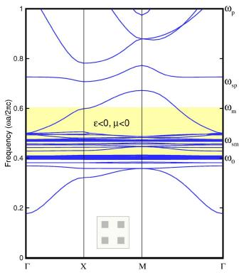
FIG. 7. (Color online) The TM band structures for a square array of square cylinders of negative index material with half-width w/a=0.2, where  $\omega_p a/2\pi c=1.0$ ,  $\omega_0 a/2\pi c=0.4$ , and F=0.56.
