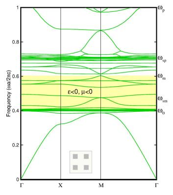
FIG. 8. (Color online) The TE band structures for a square array of square cylinders of negative index material with half-width w/a=0.2, where  $\omega_p a/2\pi c=1.0$ ,  $\omega_0 a/2\pi c=0.4$ , and F=0.56.
