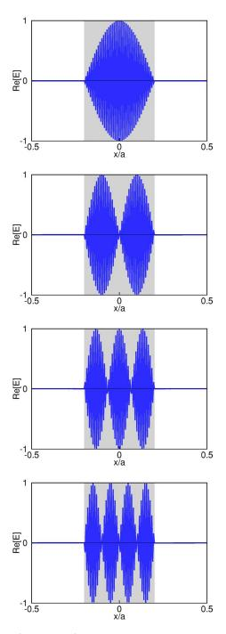
FIG. 5. (Color online) Four typical RC modes for TM polarization with  $\omega a/2\pi c=0.4$  at the zone center (k=0) with  $\beta=0$  for a one-dimensional layered structure of negative index material of thickness t/a=0.4 where  $\omega_p a/2\pi c=1.0$ ,  $\omega_0 a/2\pi c=0.4$ , and F=0.56.
