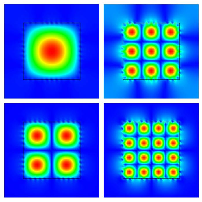
FIG. 13. (Color online) Four typical RC modes in magnitude for TM polarization with frequencies near  $\omega_0$  at the point  $\Gamma$  for a square array of square cylinders of negative index material of half-width w/a=0.3 where  $\omega_p a/2\pi c=1.0$ ,  $\omega_0 a/2\pi c=0.4$ , and F=0.56.
