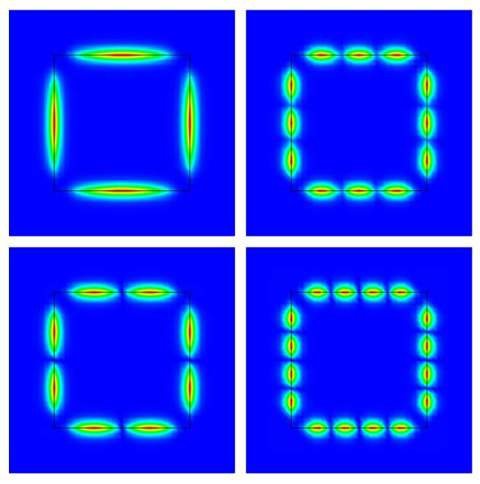
FIG. 12. (Color online) Four typical MSP modes in magnitude for TM polarization with frequencies near  $\omega_{sp}$  at the point  $\Gamma$  for a square array of square cylinders of negative index material of half-width w/a=0.3 where  $\omega_p a/2\pi c=1.0$ ,  $\omega_0 a/2\pi c=0.4$ , and F=0.56.
