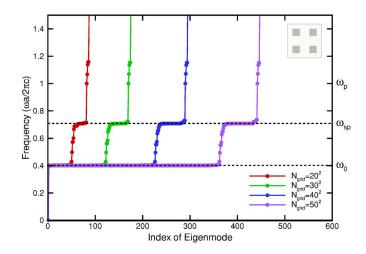
FIG. 6. (Color online) The eigenfrequencies for TE modes versus the index of eigenmode computed with different grid resolutions at the point  $\Gamma$  for a square array of square cylinders of half width w/a=0.2 where  $\omega_p a/2\pi c=1.0$ ,  $\omega_0 a/2\pi c=0.4$ , and F=0.56.
