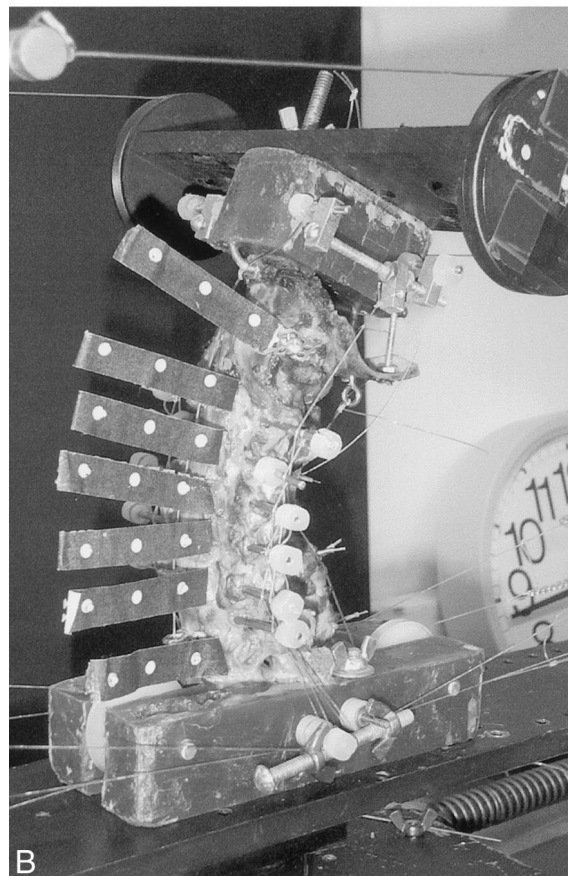
Figure 4. Flexibility testing of the specimen with MFR. A , Schematics showing the flexibility set up, where the specimen is loaded with pure flexion and extension bending moment during flexibility testing. B , Photograph of the specimen with the MFR system.
