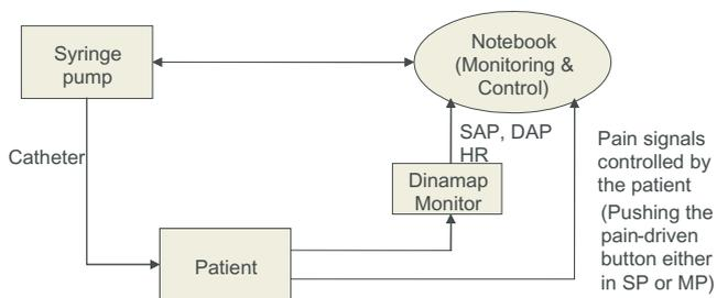
**Fig. 4** The diagram of a PCA+SLFLC controller where the control system administers alfentanil infusion depending on button-pressing profile of the patient either in severe pain (SP) or mild/moderate pain (MP).
