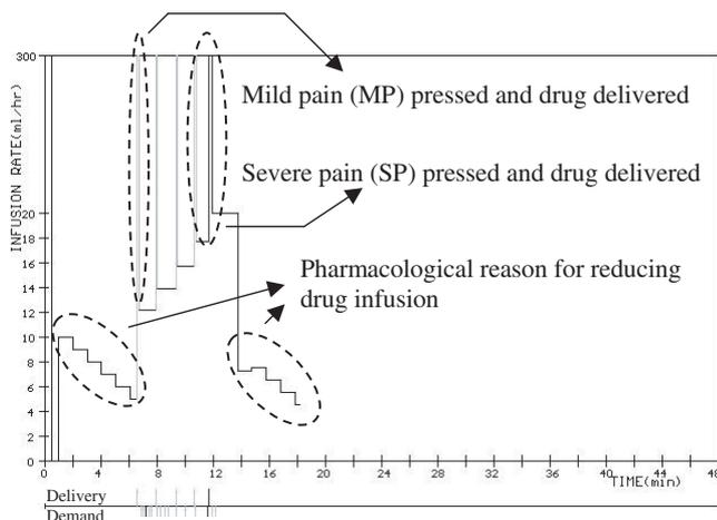
**Fig. 3** Self-learning fuzzy logic control of pain intensity for patient 10 in group B. The solid line is for alfentanil infusion rate, the heavy solid line of bolus is for SP, and the thin solid line of bolus is for MP. The demand and delivery are recorded at the bottom line (i.e. above the line is for delivery and below the line is for demand).
