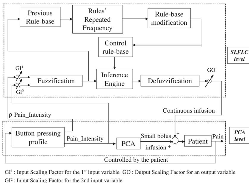
**Fig. 2** The diagram of the control system administers alfentanil infusion depending on button-pressing profile of the patient using a PCA+SLFLC algorithm.
