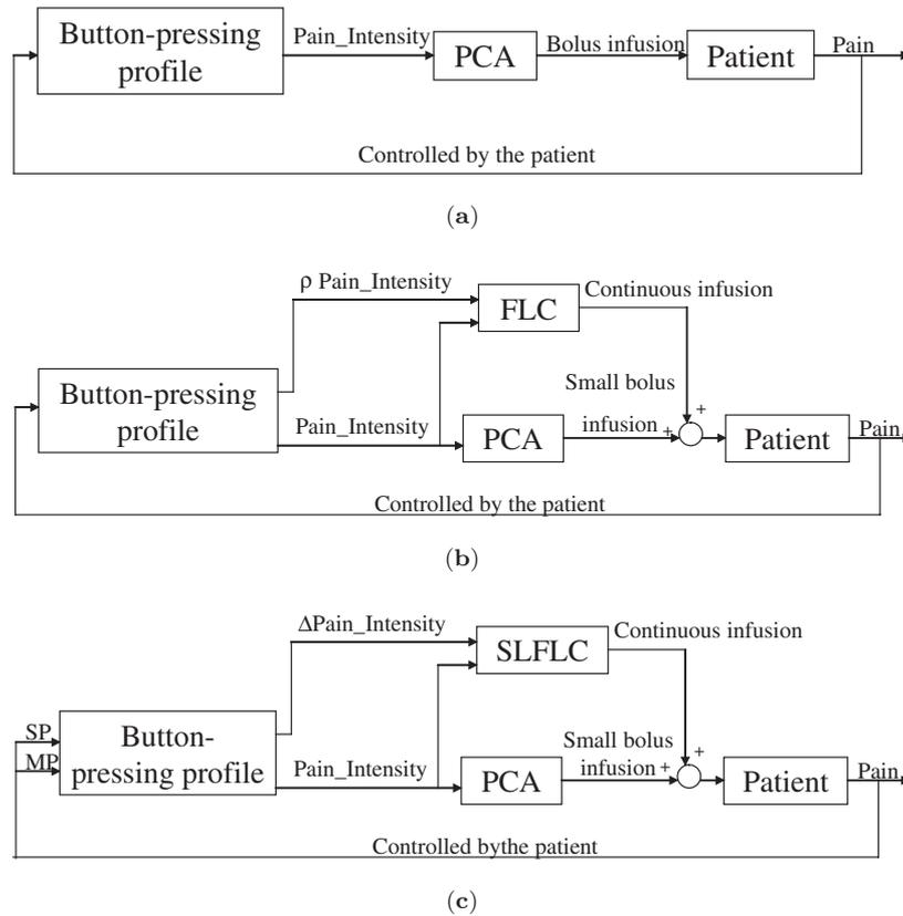
**Fig. 1** The diagrams of the control systems administer alfentanil infusion depending on button-pressing profile of the patient. (a) Conventional PCA controller; (b) PCA+FLC controller, (c) PCA+SLFLC controller.
