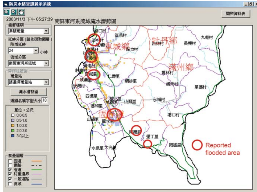
Figure 11. The inundation potential map selected by the decision support system and the reported flood area of south Pingtung County during the Typhoon Melor event.
