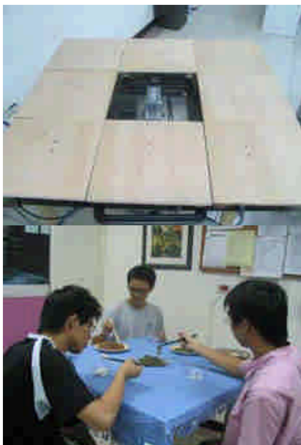
Fig. 6. The picture on the left shows the embedded RFID and weighing table surfaces, and the picture on the right shows a dining scenario.
