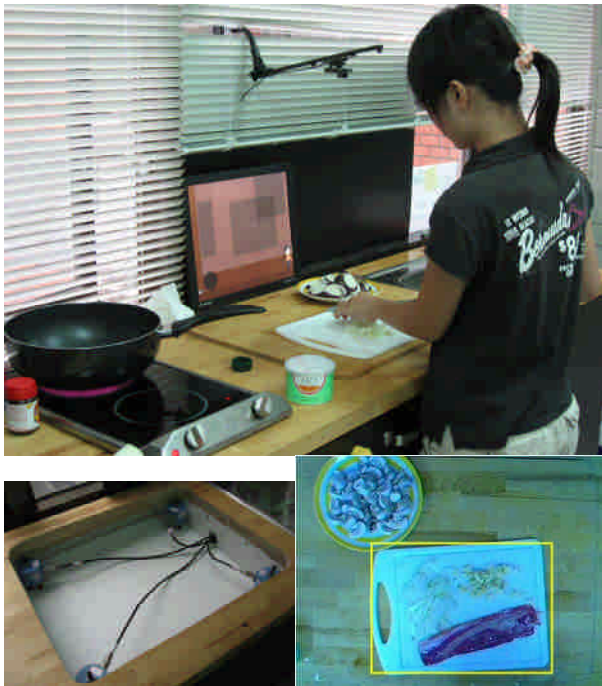
Fig. 5. Calorie-aware Kitchen with calorie tracking and digital feedbacks of nutritional information during cooking process. The bottom left shows weighing sensors deployed under counter, and the bottom right shows the overhead camera to capture images of the counter.
