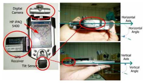
Figure 5: The HP iPAQ 5550 with camera, GPS receiver, and a Tilt sensor
