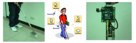
Fig. 3. In iCane, he standard white cane is equipped with a PDA, an antenna, Bluetooth headset and an RFID reader.
