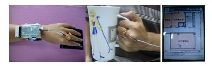
Fig. 4. The object reminder system. On the left shows the wearable wristband device. In the middle shows the RFID tag on the object. On the right is a map display showing the locations of objects.
