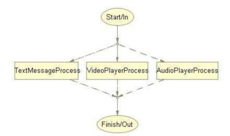
Fig. 8. Process Graph of Smart Alarm Clock
