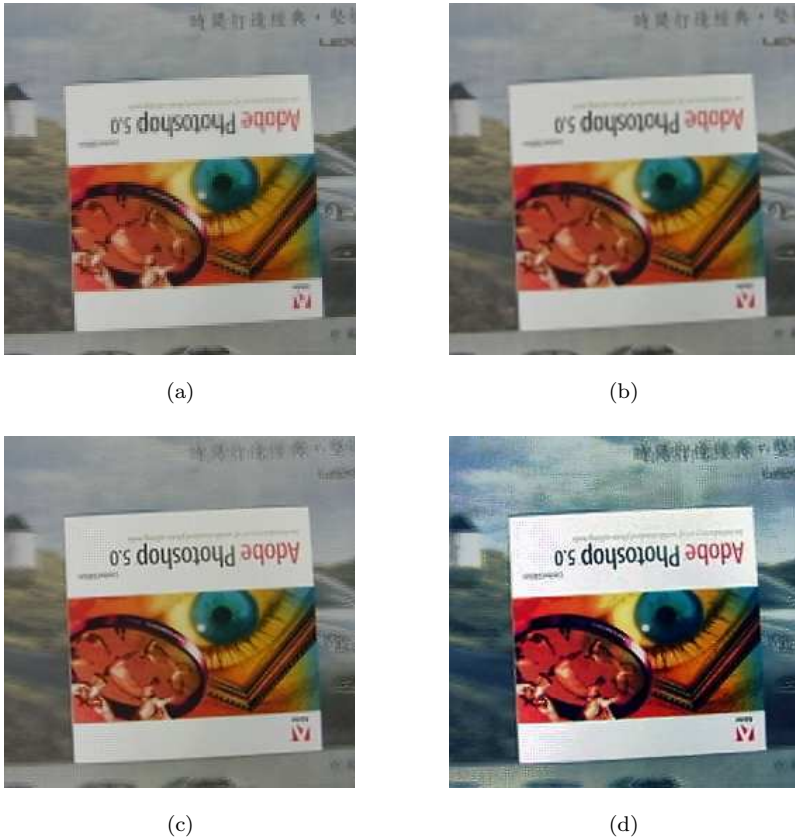
Fig. 8. Results of our proposed method with a moving scene and a fixed real camera. (a) One of low-resolution images. (b) Initial guess. (c) Reconstructed image after 100 iterations. (d) Enhanced final output image.
