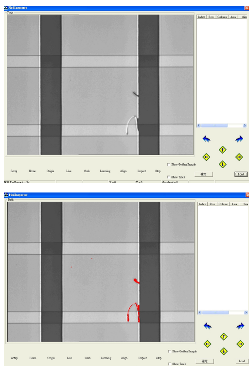
Figure 18 Inspected image (upper) and inspection result (lower).
