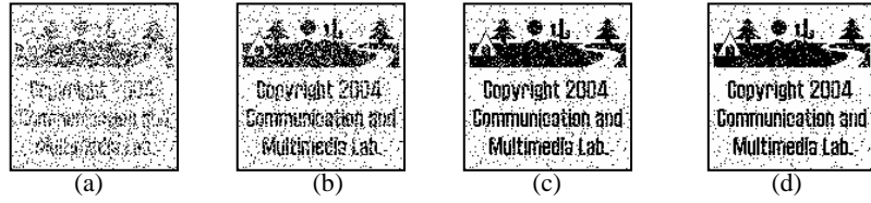
Fig. 7. Extracted watermark patterns after performing (a) 1 generations, (b) 100 generations, (c) 10,000 generations and (d) 1,000,000 generations of optimization computations, given that the pre-specified PSNR requirement is 36dB, are listed for visual evaluation.
