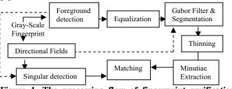
Figure 1. The processing flow of fingerprint verification system.
