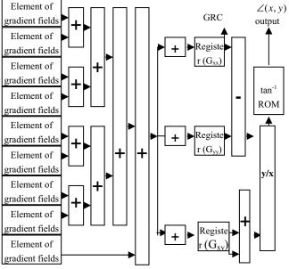
Figure 8. The gradient fields and GRC hardware architectures.
