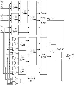
Figure 7. The thinning hardware architectures.
