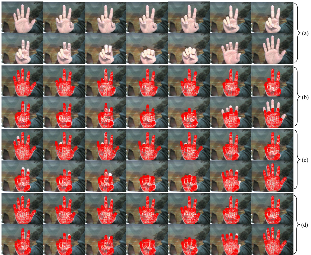
Figure 4. Five-finger tracking with 20 DOFs. (a) Input sequence. (b) Tracking results using classical particle filtering. (c) Tracking results using appearance information only. (d) Tracking results using our hybrid approach.
