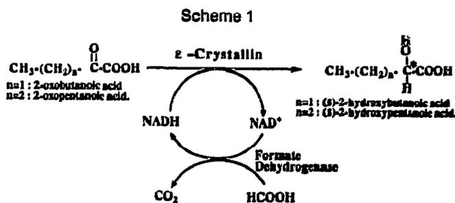
Scheme 1.  $\epsilon$ -Crystallin-catalyzed synthesis of (S)-2-hydroxy acids by an in situ NADH regeneration system coupled with formate/formate dehydrogenase.
