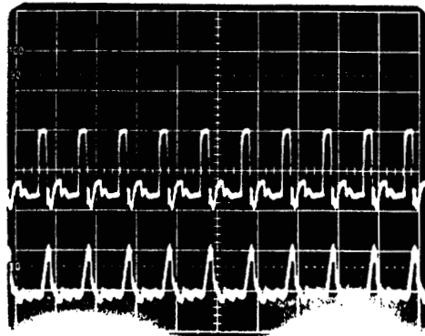
Figure 5: The output waveform (upper trace, 10 V/div) of the LED driver circuit and the received waveform (bottom trace, 0.2 V/div) from the output of the preamplifier. The horizontal scale is 1 uS/div.
