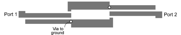
Fig. 9. Layout of the fourth-order microstrip coupled-line bandpass filter in [16].
