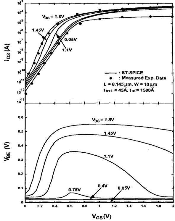
Fig. 3: (a) Drain current (b) body-source voltage characteristics of a PD SOI NMOS device biased in the subthreshold region, with its body node floating, based on the PD-SOI SPICE results, and measured data.
