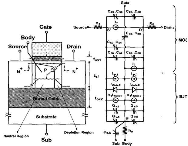
Fig. 1: Compact BiCMOS charge-control models for deep-submicron PD SOI NMOS devices used in PD-SOI SPICE.
