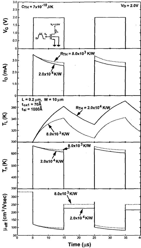
Fig. 2: Transient performance of a  $0.2\mu\text{m}$  PD SOI NMOS device in terms of drain current, lattice and electron temperatures and effective mobility, based on PD-SOI SPICE results.
