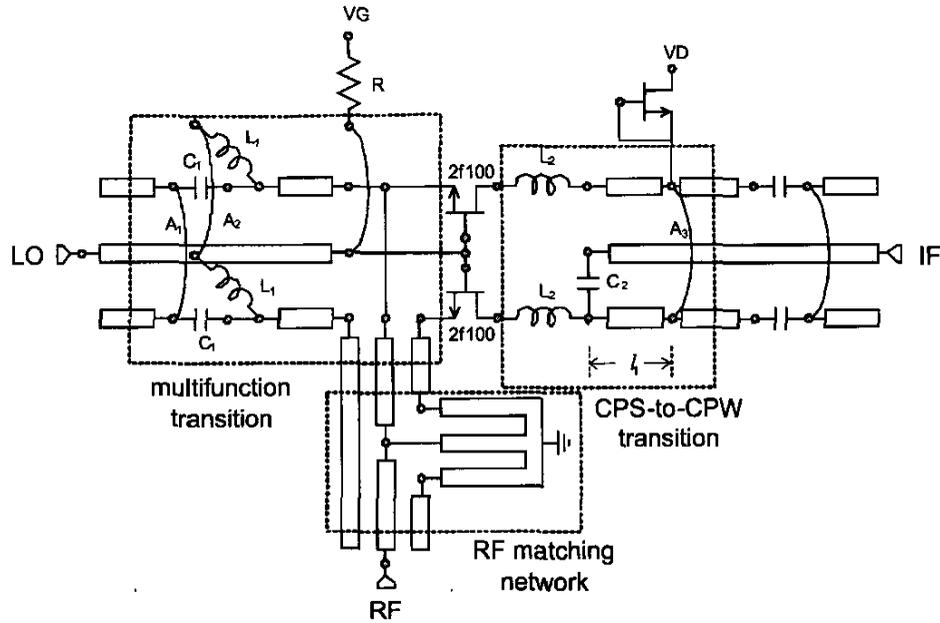
Fig. 1. Schematic of miniaturized uniplanar gate mixer.
