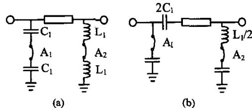
Fig. 2. Equivalent circuits of the resonant circuit operated at (a) CPS mode and (b) CPW mode.
