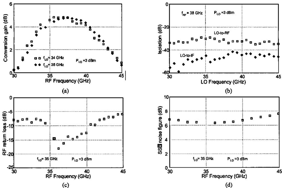
Fig. 4. Measured results for the proposed mixer (Fig. 3): (a) conversion gain, (b) LO-to-IF and LO-to-RF isolations, (c) RF return loss, and (d) SSB noise figure.
