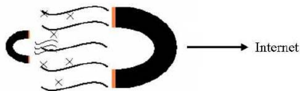
Figure 3-b. Large magnet (more resourceful sink, ex:PC) which overwhelm small magnet, attract data and transmit via wider bandwidth network (ex:ADSL) to Internet Figure 3. Resource-awareness: larger magnet out-attracting the small magnet
