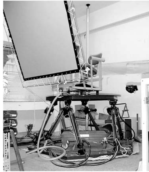
Fig. 16. Stewart platform driving simulator.
