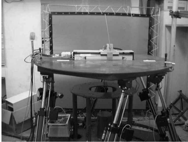
Figure 2. Photograph of the inverted pendulum system on a Stewart platform.
