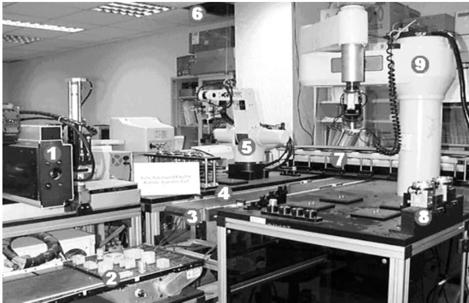
Fig. 2. Two-robot assembly cell. 1: Part loader, 2: Parts, 3: Conveyor belt, 4: Optical sensors, 5: CRS robot arm, 6: Overhead CCD camera, 7: rotatory buffer, 8: Grippers of Adept, 9: Adept robot arm.
