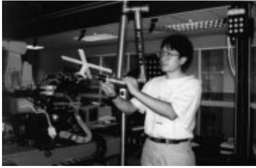
Fig. 6. Portable CMM we used for providing the initial estimates of the kinematic parameters.
