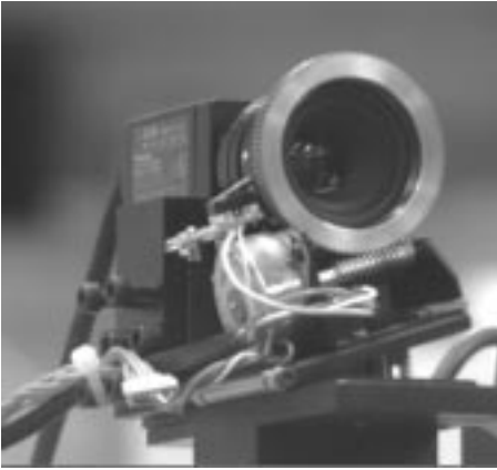
Fig. 3. Motorized lens of the IIS head.
